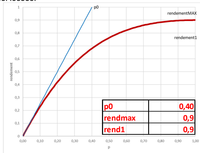
Figure 16: Only parallel losses efficiency curve
