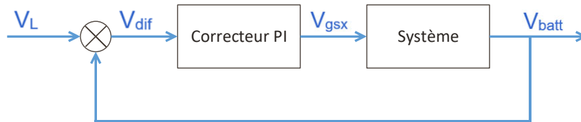
Figure 11: Simplified diagram of the regulation
